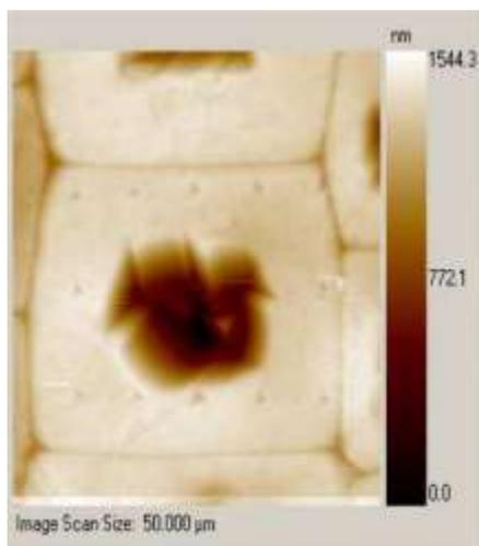
Figure. 2 Matrix of indents of summer cell wall scanned with Hysitron Tribolab®, 50 x50 μm
