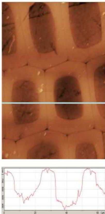
Figure 1a AFM image of a spring wood cells
