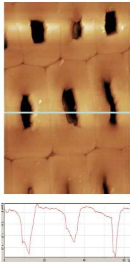
Figure. 1b AFM image of a summer wood cells
