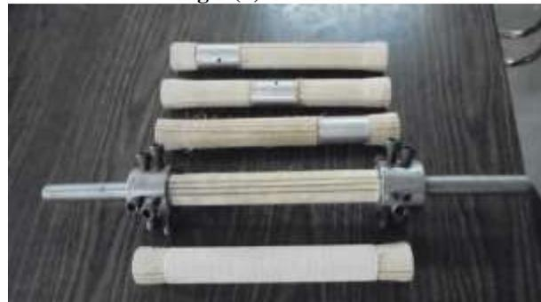
**Fig 2.(d)** Modified Specimen used for testing
