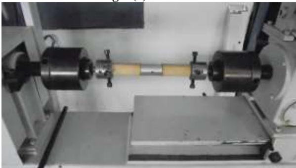
**Fig 2.(c)** Torsion test
