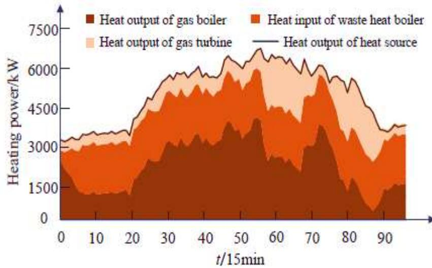
Figure 5: Optimal dispatch results of heat.
