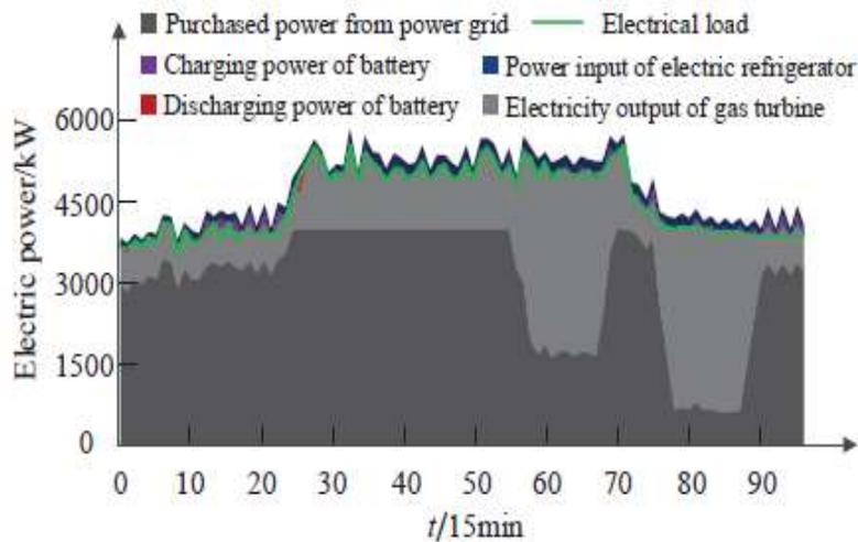
Figure 4: Optimal dispatch results of the electric power.
