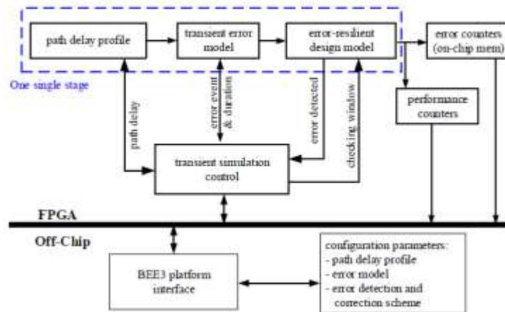
Figure 1: FPGA based transient simulator platforms. At multi stage simulations may be constructs through cascading single stage within being delay profile and model.
