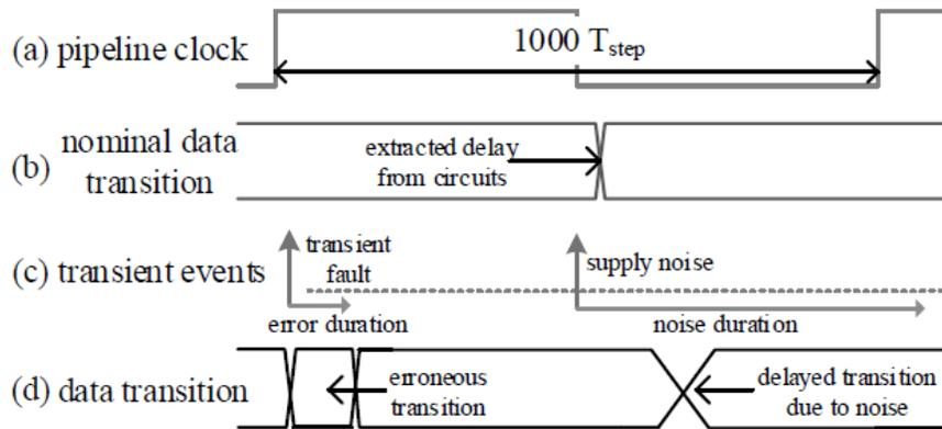
Figure 2: Timing chart to the FPGA based hardware emulations: (a) pipeline clocks, (b) extract nominal data paths delay, (c) inject transient event (error and noise), & (d) data transitions at the results with (b) and (c).
