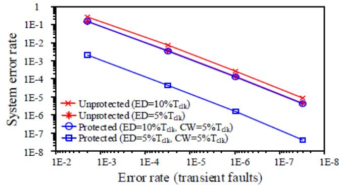
Figure 7: Reliable improvement for pre-edge errors detections and corrections (CW: checked window, ED: error durations,  $T_{clk}$ : clock periods).
