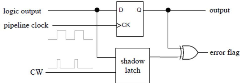
Figure 9: Post-edge errors detection circuit [5].
