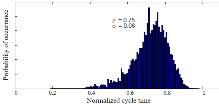
Figure 6: Simulation for delay distributions with extract CORDIC processors.
