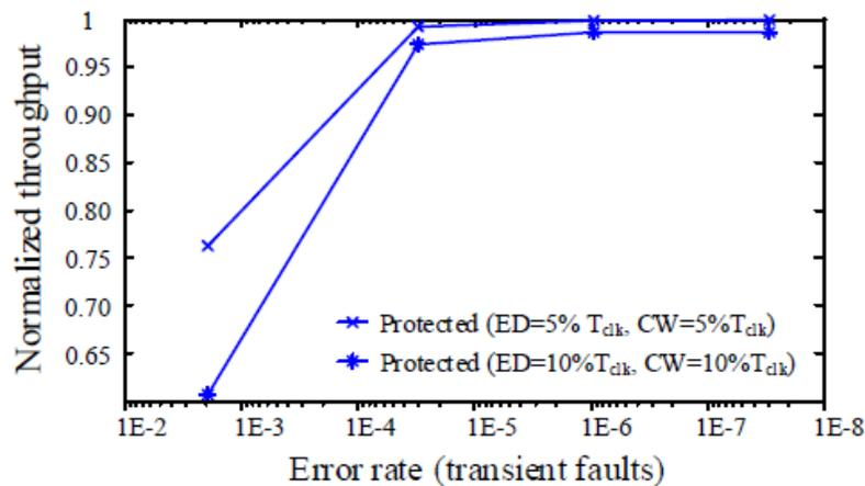
Figure 8: Effectively throughput use as pre-edge error detections and corrections (CW: checking window, ED: error durations,  $T_{clk}$ : clock periods).
