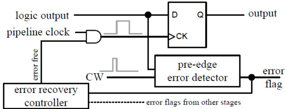
Figure 5: Pre-edge error detections & recovery between pipeline stall [4].
