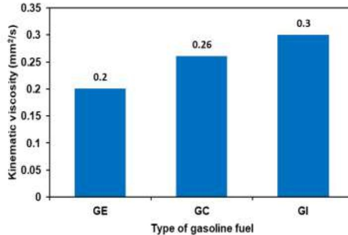
Figure 5. Viscosity for tested fuel samples
