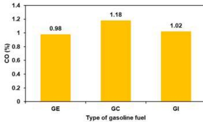
Figure 10. CO emission at 2000 rpm engine speed
