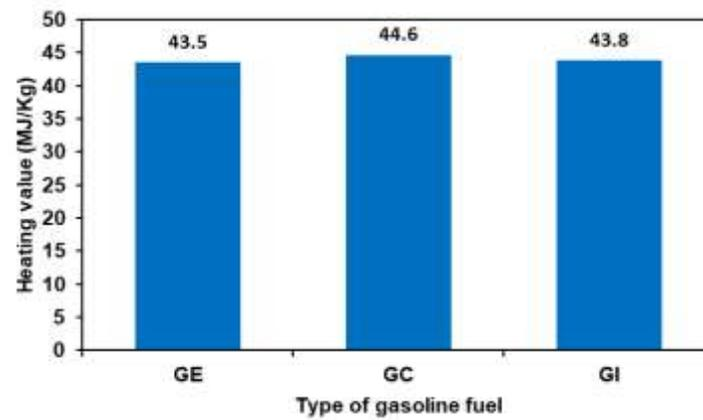
Figure 3. Heating value for tested fuel samples
