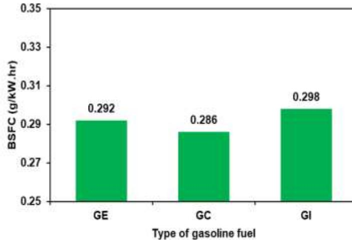
Figure 7. Brake specific fuel consumption at 2000 rpm engine speed
