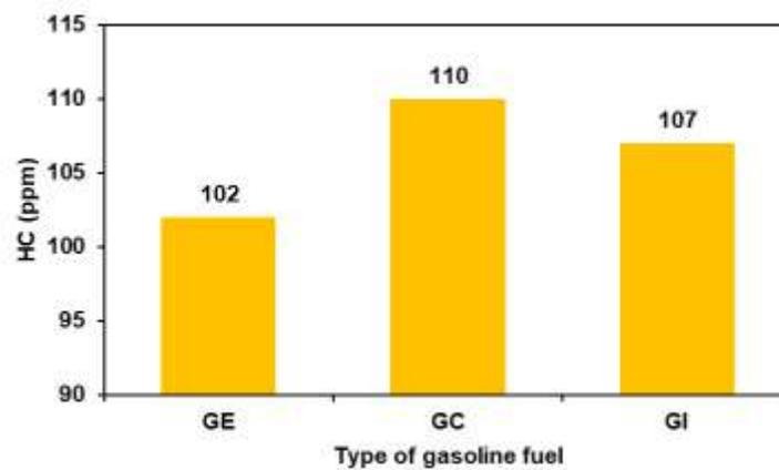
Figure 11. HC emission at 2000 rpm engine speed
