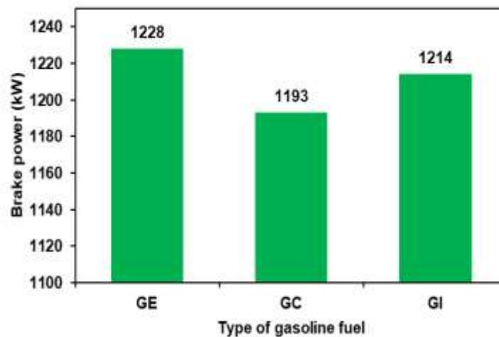
Figure 6. Brake power at 2000 rpm engine speed
