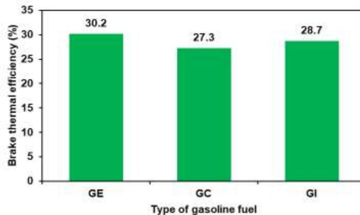
Figure 8. Brake thermal efficiency at 2000 rpm engine speed
