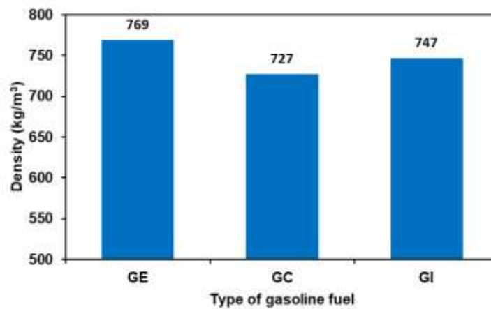
Figure 4. Density for tested fuel samples
