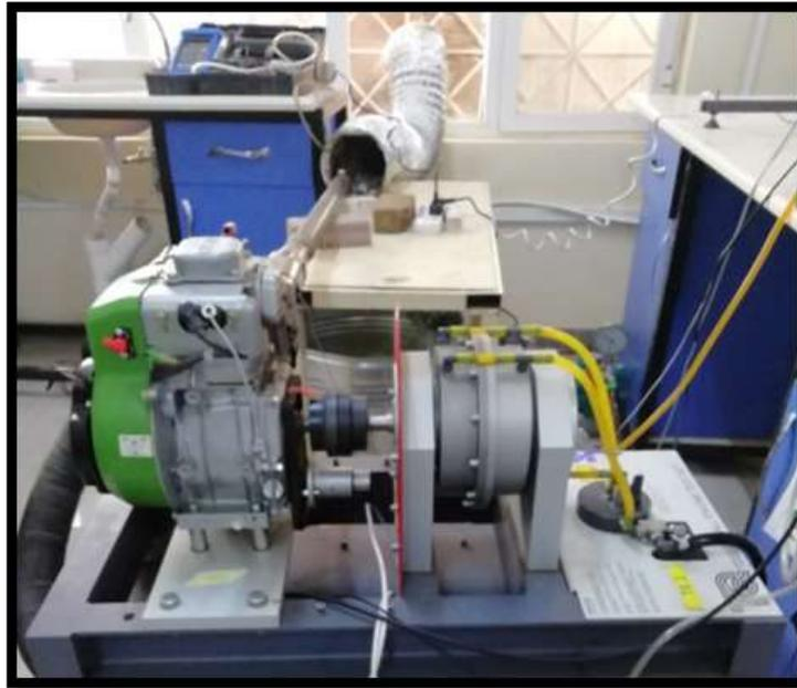
Figure 1. Engine test rig
