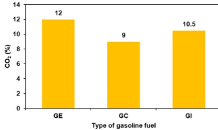
Figure 9. CO<sub>2</sub> emission at 2000 rpm engine speed
